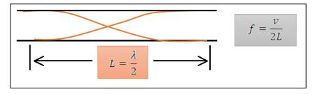
Figure 7: The fundamental or first harmonic of open resonance tube
