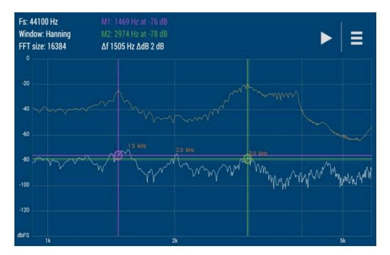
Figure 9: The experimental result and graph of 10 cm open resonance tube
