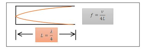
Figure 8: The fundamental or first harmonic of closed resonance tube
