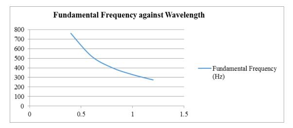
Figure 11: Graph of fundamental frequency against wavelength for closed resonance tube
