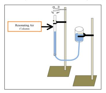
Figure 1: To determine the velocity of sound in air
